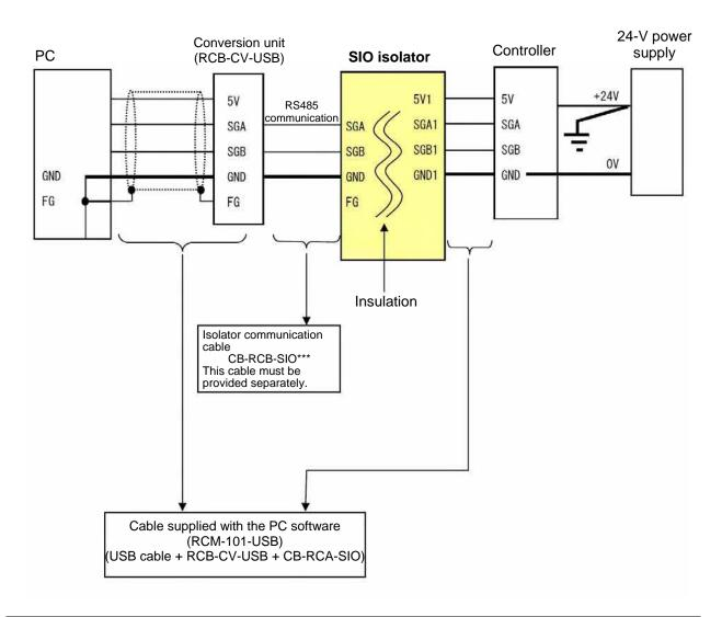
Note The RS232 conversion unit (RCB-CV-MW) cannot be used.
