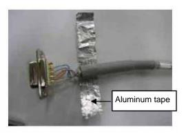
[3] Wrap an insulation table around the cable and then affix the cable with the cable holder. At this time, make sure the shielded wire does not project from the cable holder. (Cut the shielded wire, if necessary.)
