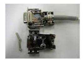
[2] Take out the cable holder and then remove the aluminum foil tape.
