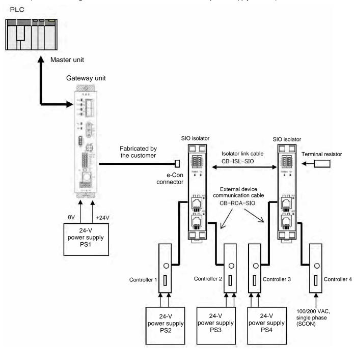
Note The power to the primary circuit in the SIO isolator is supplied from the CN1, so be sure to connect the CN1.
